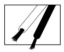
**4. A.** Cut Neon (at cutting points) to fit or join multiple sections as recommended to cover installation area.
