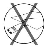
**Do not** put direct excessive pressure on the Neon LED surface.
