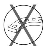
**Do not** bend Neon LED to a diameter less than 1.5 inches.
