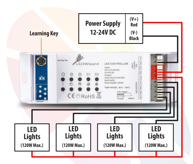
**Note:** The LEDWizard Manual Dimmer can drive up to 240W at 12V DC or 480W at 24V DC. However, each of the 4 output terminals is 5A and can only handle a maximum wattage of 60W at 12V DC and 120W at 24V DC. Do not put on one output a load (LED Fixture) that is more than the maximum wattage it can handle. If the load is more than 60W and you are using a 12V DC Power Supply, make sure to split the load and use more than one output.
