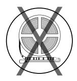
**Do not** bend LED strips to a diameter less than 1.5 inches.
