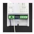
Connect the RGB fixture's wires to the "DC OUTPUT" screw terminals of the controller with Red connected to R-, Green to G-, Blue to B-, and the positive (could be black or another color) to V+.
