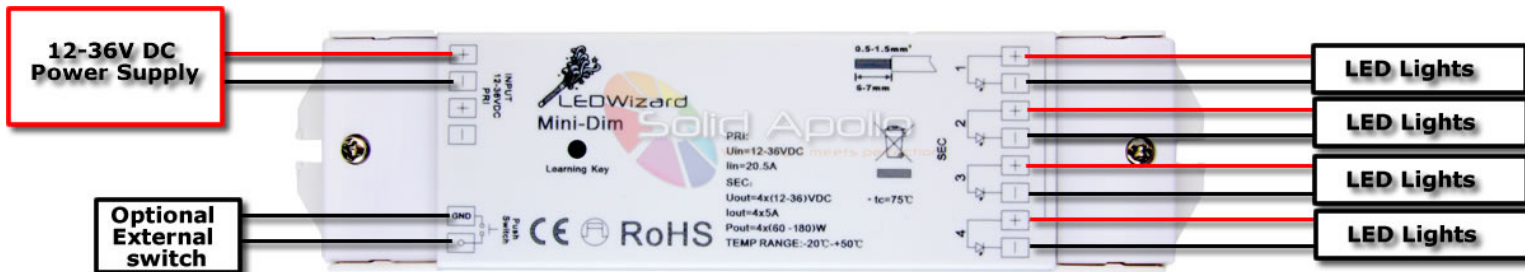
Figure 2. Wiring the “Mini-Dim” Glide Receiver
