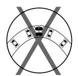
**Do not** bend LED strips to a diameter less than 1.5 inches.
