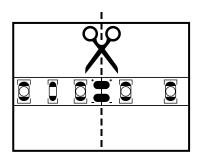
**5.** If using Channels, cut or extend them to fit size of the installation area
