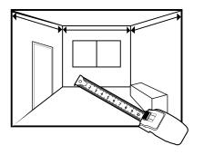
**3.** Determine how much wire needed (Driver to Dimmer, Dimmer to LED Strips).
